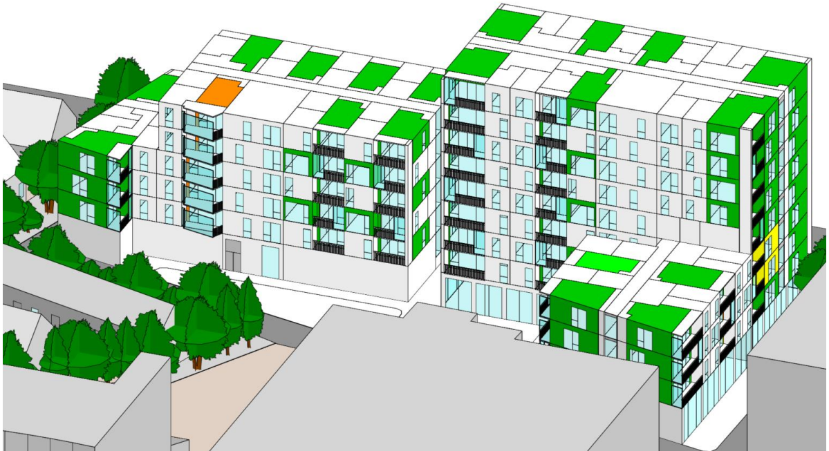
Above: Kitchen/Living space ADF results of the proposed development from the West.
