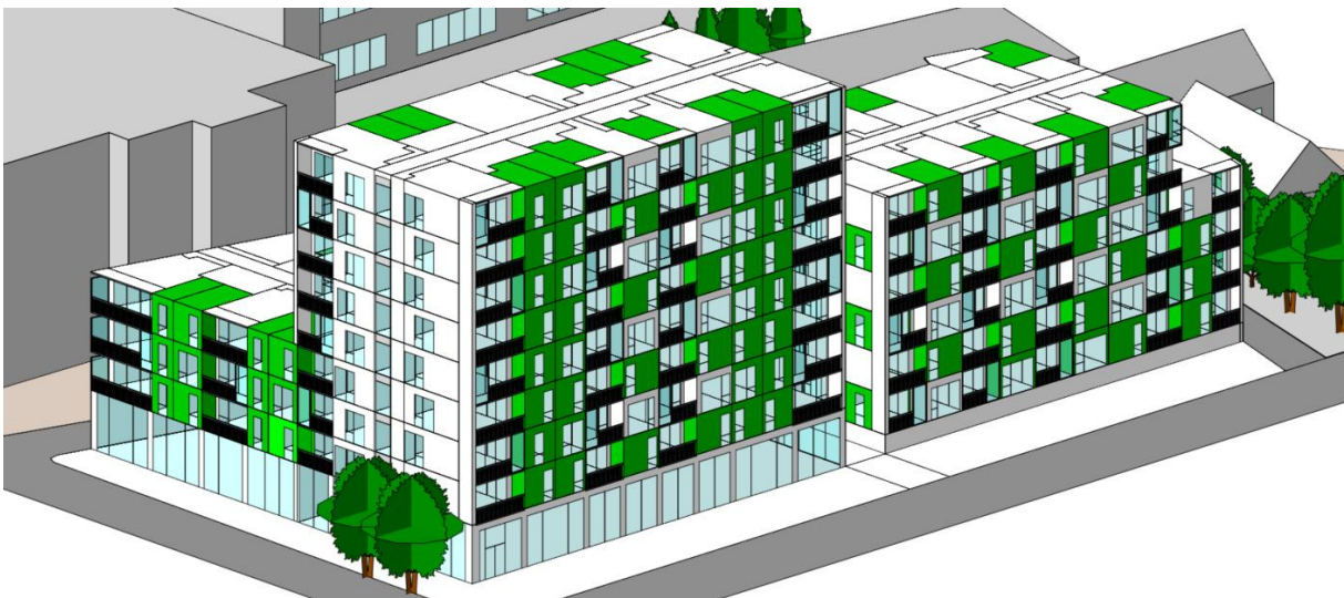
Above: Bedroom ADF results of the proposed development from the South East.
