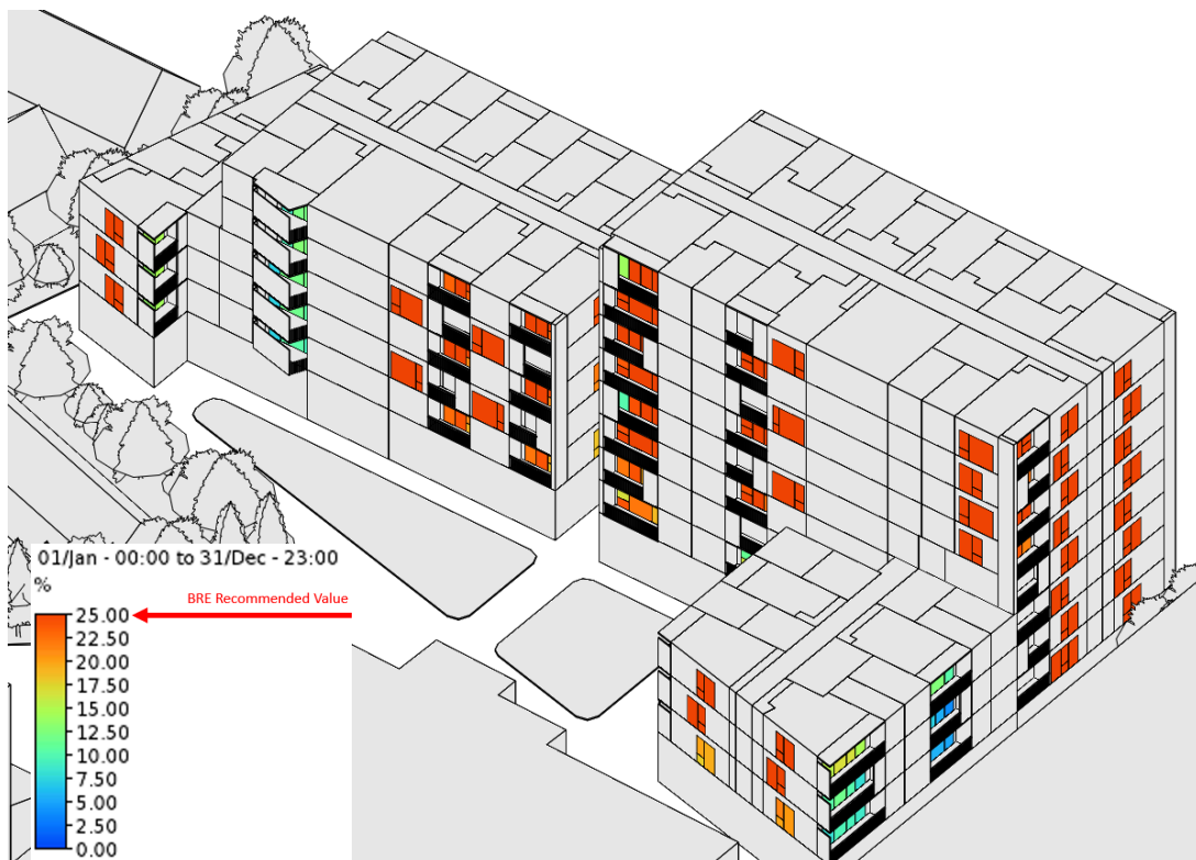
Above: The image above (taken from the south west) shows the living spaces within the proposed development that achieve 25% of their annual probable sunlight hours (highlighted in red) meaning these spaces will appear reasonably sunlit in line with BRE 209 guidance.
